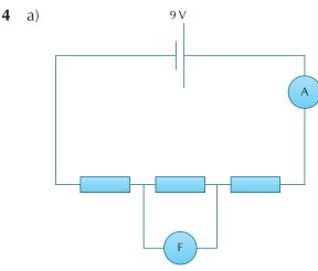
Voltmeter can be across any resistor.
