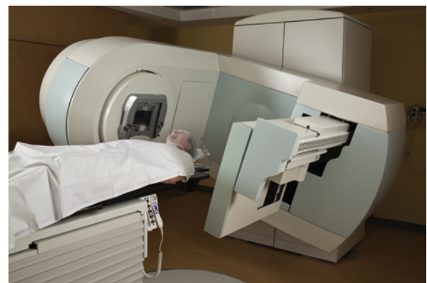
Figure 12 The rotating gantry limits the dose to healthy tissue.
