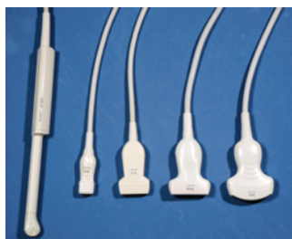
Figure 8 Ultrasound transducers of different size and shape for optimum positioning
