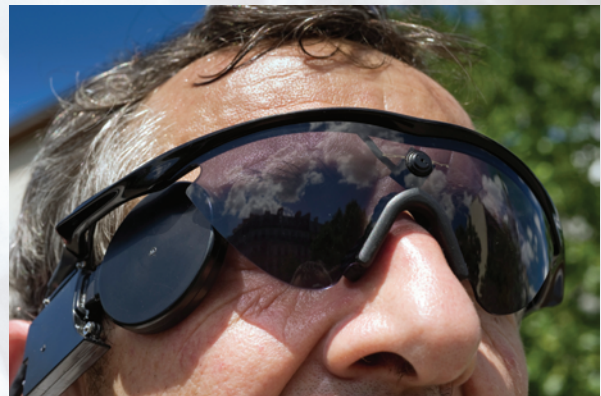
A retinal implant user. The camera is at the centre of the glasses. The box lower left is an antenna that receives signals from the VPU (worn on the body) and transmits them to the implant.
