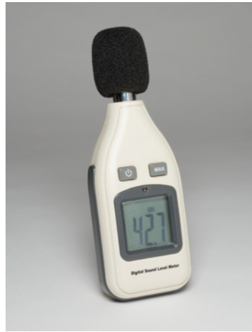
Figure 31 A sound level meter with a readout in dBA. This type of meter is used for environmental and industrial noise monitoring.
