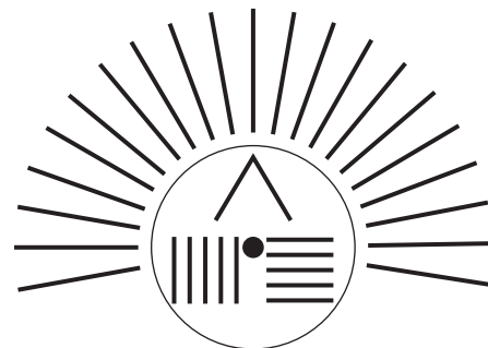
Figure 18 A person suffering from astigmatism sees some lines in this optician's chart clearer than others.
