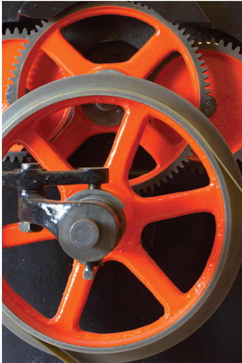
Figure 20 In a flywheel, the spokes are symmetric, for stability. Although the majority of the mass ideally needs to be at the rim, there are also structural and safety considerations to take into account.
