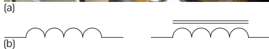
Figure 15 An inductor and its circuit symbol. The bars on the second symbol indicate that the inductor has an iron core.
