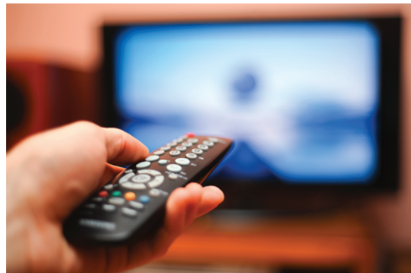
Figure 3 A TV remote control contains an infrared LED that transmits a modulated infrared signal to communicate with the TV.
