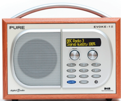
Figure 7 DAB (Digital Audio Broadcasting) is a digital radio technology used for broadcasting radio content using digital signals. This exploits the ability of digital signals having very low noise to give a pure sound on reception.
