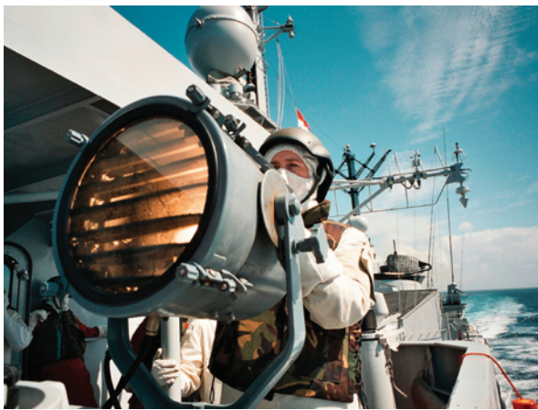
Figure 2 A signalman modulating a light signal with Morse code
