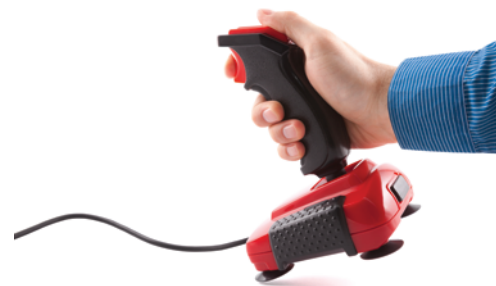
Figure 31 A joystick used in computer games makes use of the Hall effect.
