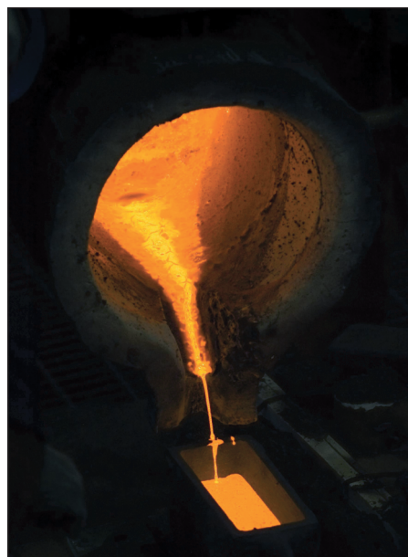
Δ Fig. 2.3 The molten iron can be poured into a mould before it cools down and turns back into a solid.
