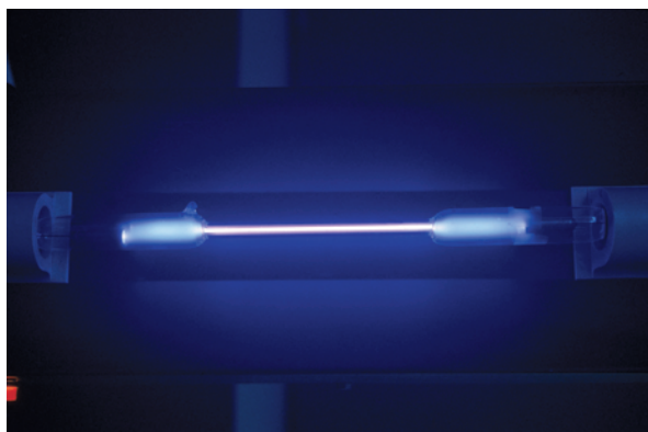
Figure 1 Lilac glow from a modern argon discharge tube
