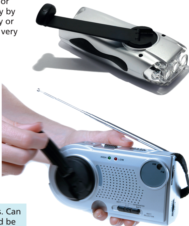
FIGURE 1.6.5b: Dynamos transfer energy of rotary motion to electrical energy.
