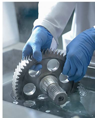
FIGURE 1.6.18c: Ultrasound was used to clean these gear teeth.
