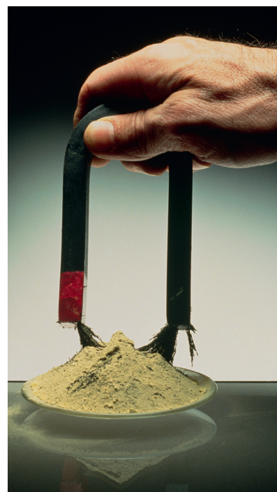
FIGURE 1.3.7b: The physical property of magnetism can be used to separate magnetic from non-magnetic materials.
