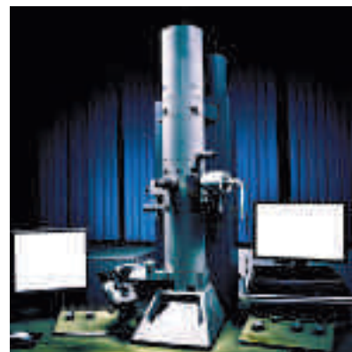
Figure 1.7 A transmission electron microscope. The electrons are displayed as an image on a fluorescent screen
