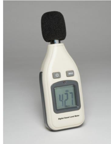
Figure 31 A sound level meter with a readout in dBA. This type of meter is used for environmental and industrial noise monitoring.
