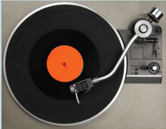
Figure 3 A vinyl record. The stylus tracks the groove inwards from the edge.
