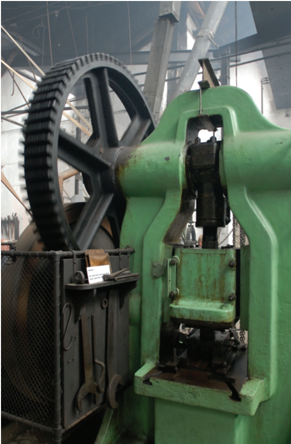
Figure 24 Punch presses are designed to cut (very regular) holes in material, so precision and consistency are essential. A flywheel, as can be seen in this old punch press, ensures that this happens.
