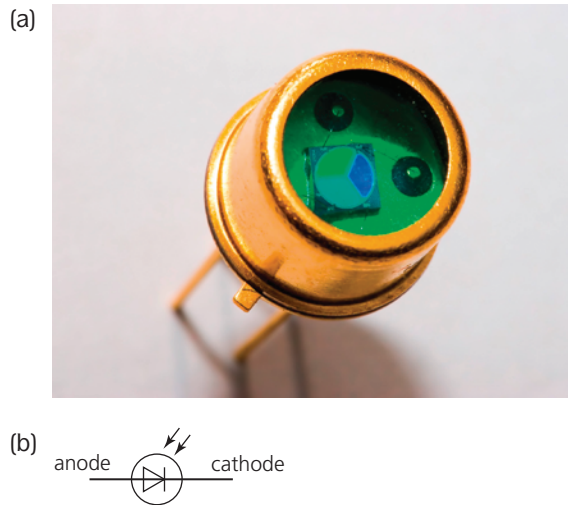
Figure 18 Photodiode and its symbol. Note that sometimes the circle in the symbol is omitted.
