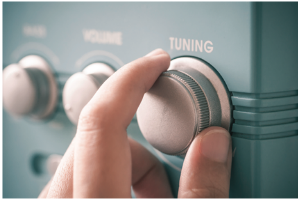
Figure 13 Tuning in to a radio station involves using a filter circuit, which filters out all frequencies except that of the broadcasting station frequency.
