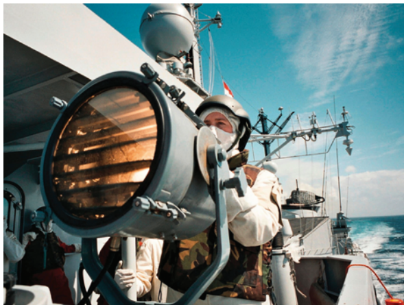
Figure 2 A signalman modulating a light signal with Morse code
