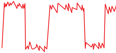
Figure 6 A noisy digital signal. Despite the noise, the pattern of high–low states can still be recognised.
