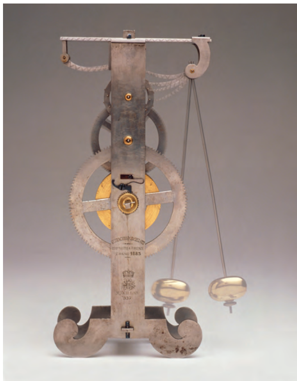
Figure 10 A model of Galileo's proposed design for a pendulum clock. Galileo realised that a swinging pendulum could be used for time-keeping. This was a major step in the history of the development of clocks.
