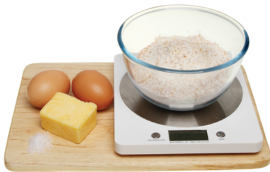
Figure 9 Finding a difference in two quantities, for example finding the mass of sugar in a bowl, can lead to large percentage uncertainties.
