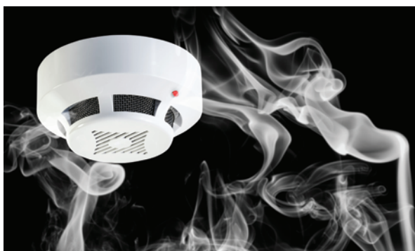
Figure 23 There is a small amount of a radioactive isotope in a smoke detector. This causes the air inside to be ionised. A small electric current flows across an air gap. When large smoke particles enter, they interfere with the current, causing the alarm to sound.
