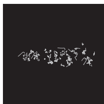
Figure 25 This cloud chamber photograph shows the ionisation caused by a gamma ray. Most of the tracks are made by secondary electrons, knocked out of their atoms by the gamma ray.
