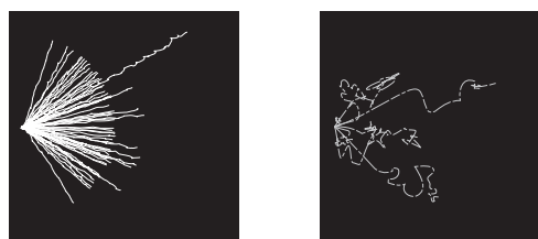
Figure 20 Tracks of alpha radiation (left) and beta radiation (right) in a cloud chamber
