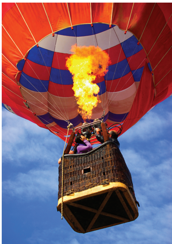
Figure 6 Balloon rides today use hot air and work on the principle that air expands and becomes less dense.
