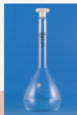
Figure P2 Volumetric flasks come in a range of sizes. The graduation mark is on the neck of the flask. The temperature for which it is graduated is also shown on the flask.
